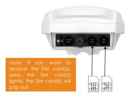
Note: The number of SIM cards to be used is dependent on the router installed in the CPE. If one SIM card is used, make sure you use the correct SIM extender connected to your router.
